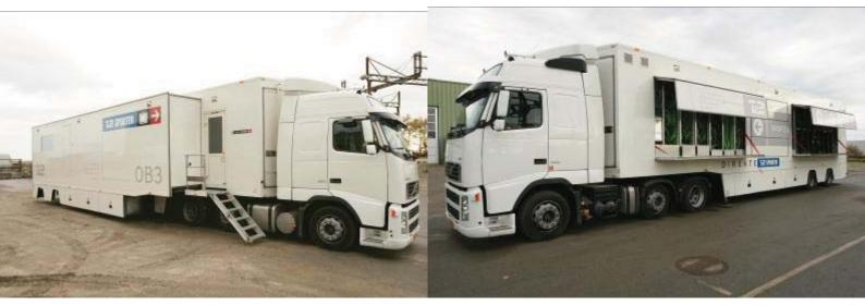
Megaspace L Trailer used as mobile TV Transmission Unit. It carries own internal power supply and A/C. Fully equipped with computers and 30+ TV screens to control transmissions from any location. This trailer has more than 400 km of cables.
