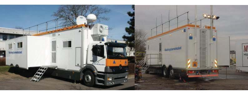
Multispace L Truck used as Command & Control Unit by the Danish Civil Defense. It carries own internal power supply, A/C and floor heating. Fully equipped with modern telecommunication systems, TV screens and computers this unit is ideally suited for the role as a mobile command station. The unit is on constant alert as a part of the Danish Civil Defense organisation in emergencies and catastrophic events.
